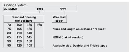
Specifications from 70°C - 160°C Standard operating temperature range in 5K steps ± 10K Tolerance on open temperature Max. Ambient temperature 175°C 20K minimum Differential
