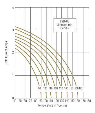
These curves are to be used only as a guide in selecting a protector for a particular application. Factors such as distance from the heat source and the method of mounting should be considered in selecting a protector. Final trip times are dependent upon terminal configuration and mounting in the application
