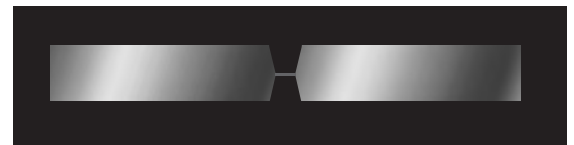
Fig. 2 Silver link semiconductor fuse.
